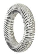
The Bal Spring® canted coil spring is a versatile component that mechanically fastens, conducts electricity, and shields sensitive electronics from the harmful effects of electromagnetic interference (EMI), and radio-frequency interference (RFI). The spring's independent coils, which serve as multiple contact points for optimal current carrying capability in electrical and shielding applications, ensure consistent, reliable connection—even under shock and vibration.
