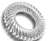
The solutions we develop begin with proven Bal Spring technology. In electrical conducting and EMI/RFI shielding applications, the spring's individual coils provide multi-point contact, and they compensate for mating surface irregularities and misalignment. As a contact component, the spring offers superior conductivity and power density. It runs cooler than other contact technologies, and it is also self-cleaning.
