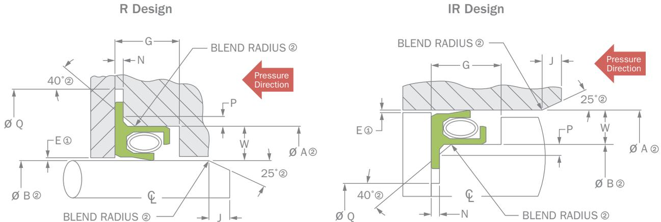
①Radial clearance determined by service conditions (a recommended radial clearance is shown on Bal Seal Engineering design proposal drawings; refer to page 21 for radial clearance dimension). ②Refer to page 22 for recommended surface finishes.
