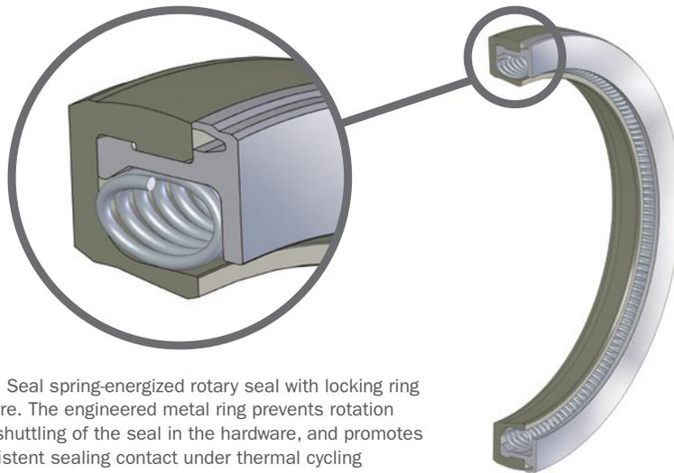
A Bal Seal spring-energized rotary seal with locking ring feature. The engineered metal ring prevents rotation and shuttling of the seal in the hardware, and promotes consistent sealing contact under thermal cycling conditions.
