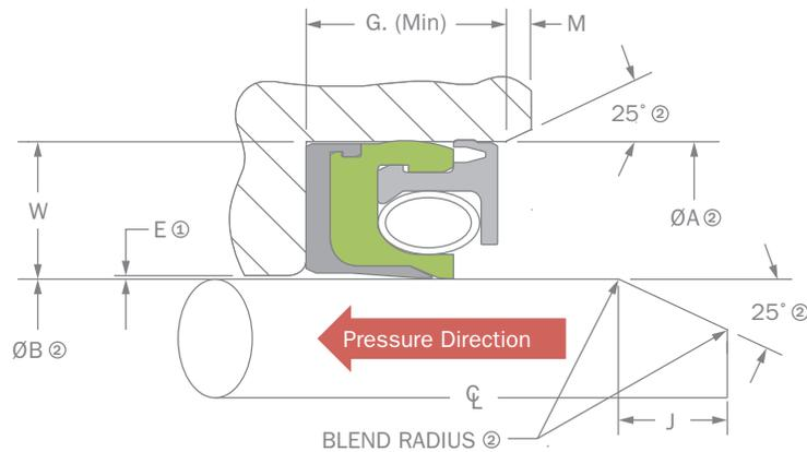
①Radial clearance determined by service conditions (a recommended radial clearance is shown on Bal Seal Engineering design proposal drawings; refer to page 21 for radial clearance dimension).
