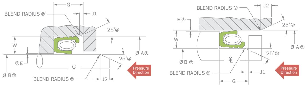
①Radial clearance determined by service conditions (a recommended radial clearance is shown on Bal Seal Engineering design proposal drawings; refer to page 21 for radial clearance dimension). ②Refer to page 22 for recommended surface finishes.
