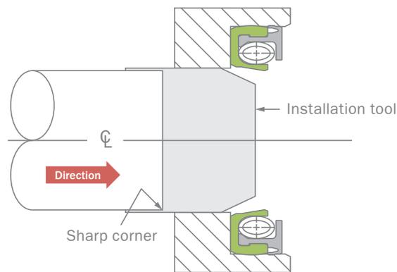
Assembly of shaft from forward direction
