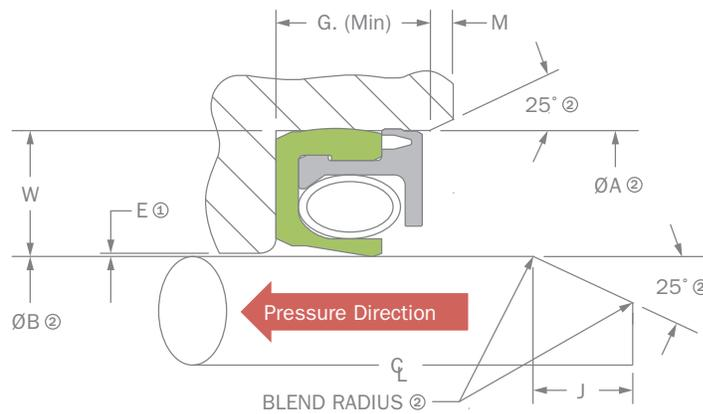
①Radial clearance determined by service conditions (a recommended radial clearance is shown on Bal Seal Engineering design proposal drawings; refer to page 21 for radial clearance dimension).
