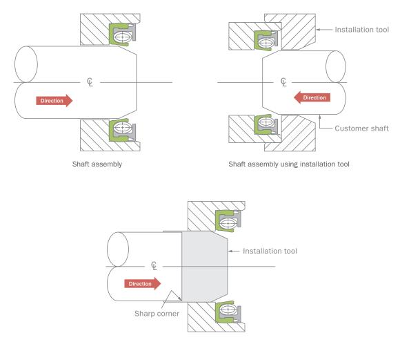
Assembly of shaft from forward direction
