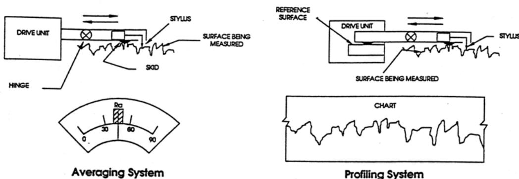
Surface Finish Measuring Instruments
