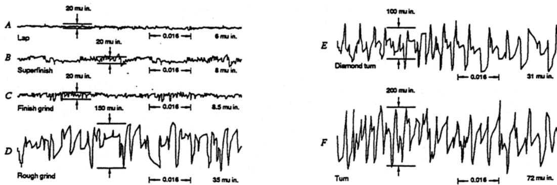
Profile Recordings of Various Machined Surfaces
