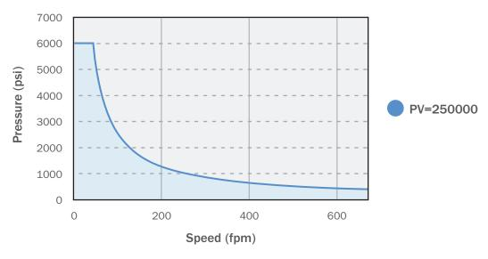
Effective sealing in high pressures and speeds is a balancing act. Designers should target a PV value of 250,000 or less in order to ensure optimal equipment service life.
