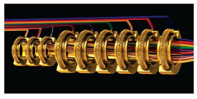
Bal Spring canted coil springs reliably conduct isolated current and signals along connectors and through tool strings in high shock/vibration environments.
