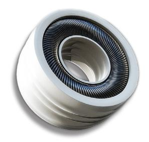
Bal Seal® spring-energized seals are made from speciallyformulated polymers, such as virgin and blended PTFE, UHMWPE and PEEK. In addition, Bal Spring® canted coil spring energizer types can be paired with seal materials to meet exacting application requirements and provide longer service life.
